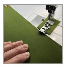
Sew until you come to the end of the row of stitching, then sew off onto a scrap fabric here as well. This is because the coverstitch does not "chain off" the same way that an overlock stitch does. By sewing off onto a scrap fabric, you'll keep your stitching intact and won't potentially need to rethread the machine before you start sewing the next row.
