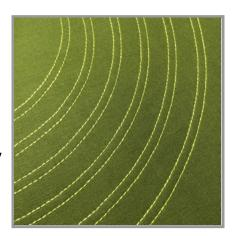
Select "Coverstitch, Wide" which is Stitch #24 on your machine screen. Your PFAFF® admire™ air 7000 coverlock machine will set the optimum thread tension, stitch length, and differential feed for your selected stitch.
