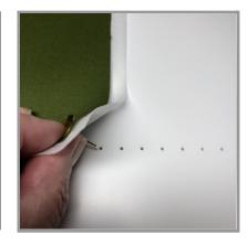
To check your stitch after initial threading, it is helpful to leave the tails of the needle threads fairly short - about 2" (5cm) long - so they can quickly pass through the needle holes of the presser foot before you start sewing your main fabric. Bring your main fabric in front of the presser foot and continue stitching.
